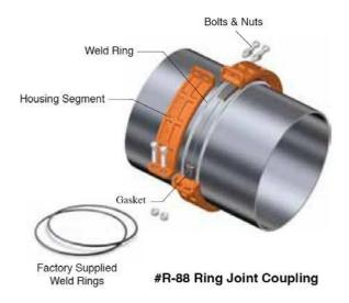
First weld a factory supplied weld-on ring on each pipe end. Next mount the rubber gasket over the pipe ends and place the coupling segments over the gasket and fasten the bolts and nuts. The same C-shaped style gasket as used in the grooved system effectively seals the pipe ends. Rings can be welded in the fabrication shop or in the field and the coupling housings can be installed on the job site.
